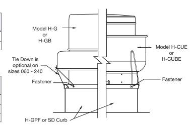
Fasteners on each side of the fan are to be installed with one fastener 4 inches (102 mm) from each edge and one fastener centered. The remaining fasteners are to be equally spaced.
